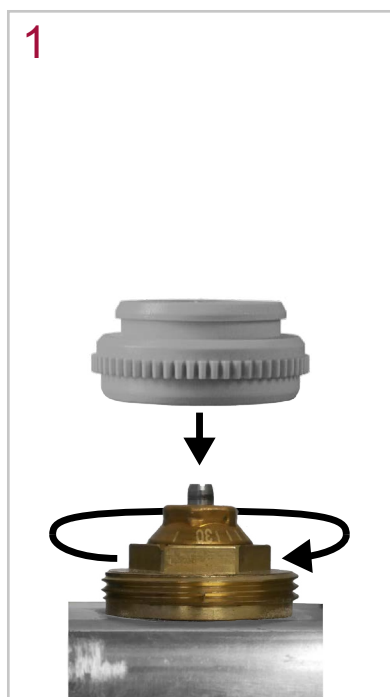
First, the valve adaptor is screwed onto the manifold valve
