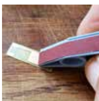
Step 2 Clean the probe
